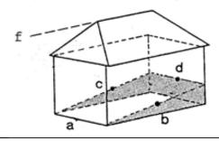
a, b, c, d = avg finisthed grade on each building wall Average Grade (entire building): (a+b+c+d)/4 = e Height = f (elevation at peak) – e (average grade)
